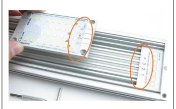
Select the module position and insert (but do not press in yet) the module. **Make sure the polarity is properly aligned:**
