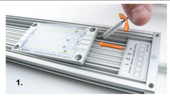
Lift and remove the module in two steps: Insert the short, rubber shank of the special key tool into the thread grooves and lever out the module.
