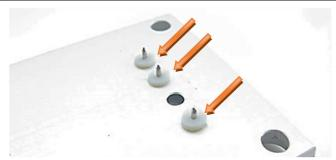
Depending on the version, the modules can have from 2 to 4 contact pins (on the bottom). All pins must be fitted with a seal. Modules with damaged or missing seal gaskets must not be used.
