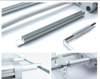
The adapter rods are graduated at one side and have a rubber bumper. These can be used for support (e.g. directly at the tank edge or on one partition of the cover).
