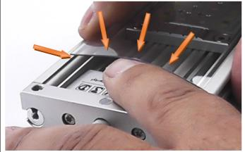
**2.** Bend the end of the panel in a slight arc; insert it into the opposite profile groove.
