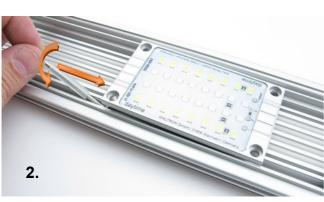
NOTICE! The rubber part must be on the short shank of the key tool. It must also cover the key edges completely so that it does not damage the bottom of the module.
